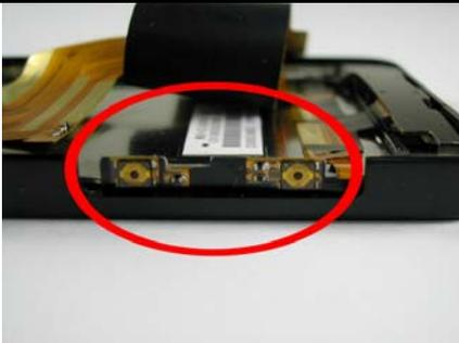
1. CONNECT THE MAIN FPC CONNECTOR TO THE NAVI BOARD, STICK THE FPC AND TIGHTEN THE MAIN FPC SCREWS AT THE LOCATION INDICATED (P/N: 72H02450-00M).
