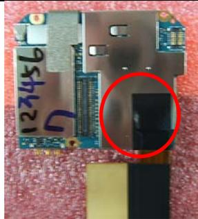
1. CONNECT THE I/O BOARD CONNECTOR TO THE M/B
